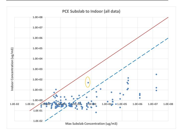
**Figure 33**Tetrachloroethene Attenuation Across the Building Envelope. (Red line is an attenuation factor of 1, Blue Line corresponds to an attenuation factor of 0.01) *NESDI Vapor Intrusion Project*
