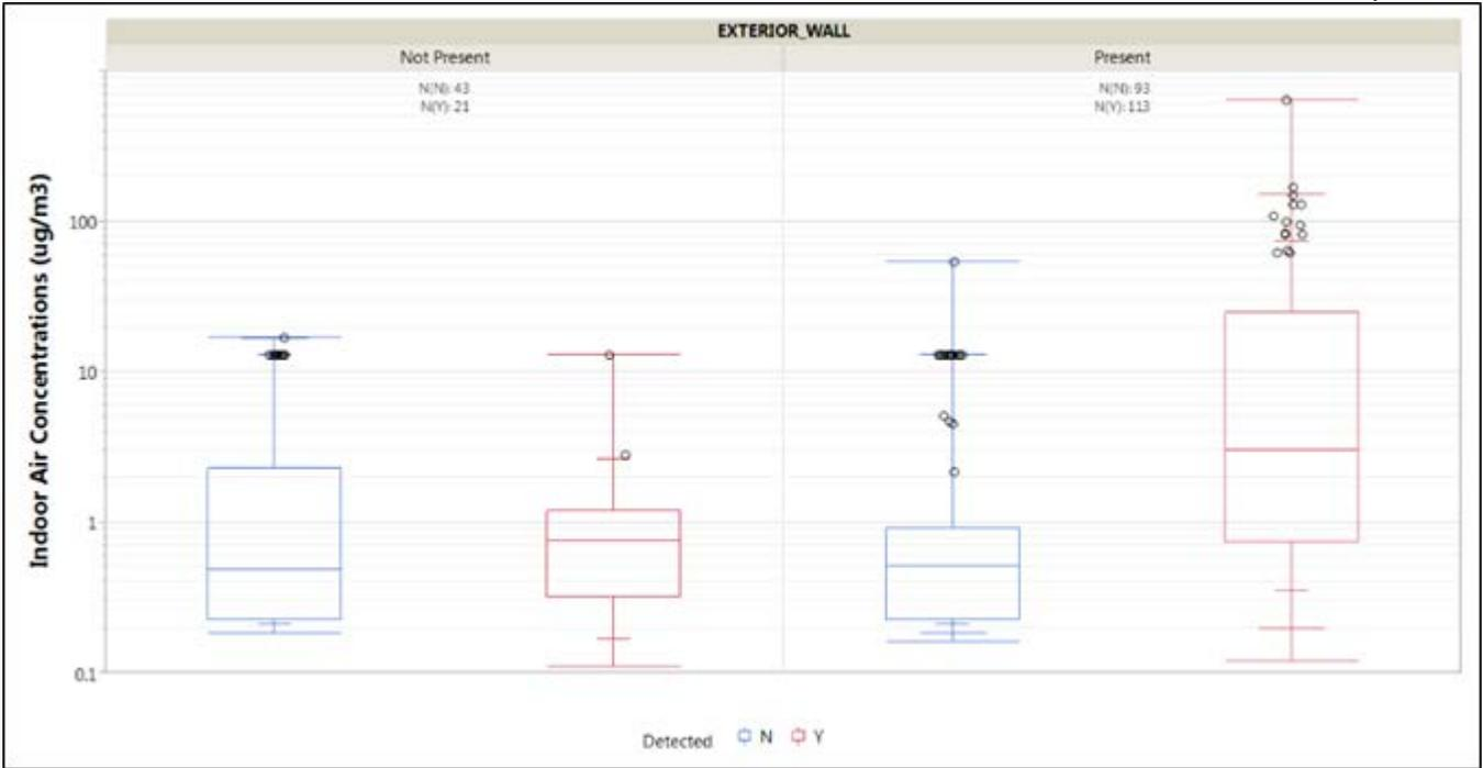
Figure 6-35. TCE Box and Whisker Plot of Indoor Air Concentration vs. Exterior Wall Presence in Sample Zone
