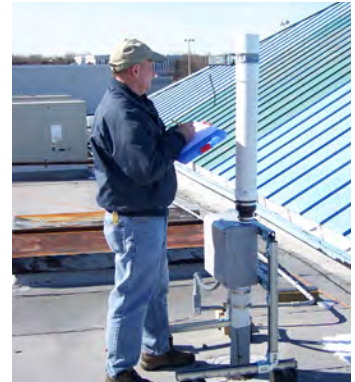
Figure 9. Blower exhaust airflow performance testing for total system.
