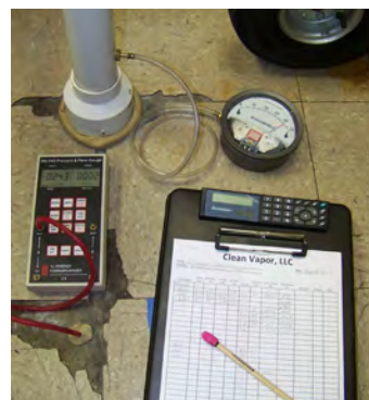
Figure 4. Static vacuum test.
