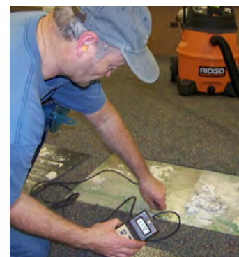
Figure 5. Measuring sub-slab vacuum.
