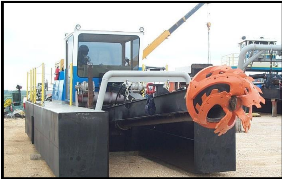
Figure 4-7. Raised Cutterhead on Land (Source: Battelle, 2010)
