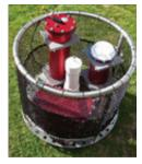
Figure 1. UltraSeep Meter (Source: NAVFAC, 2017)
