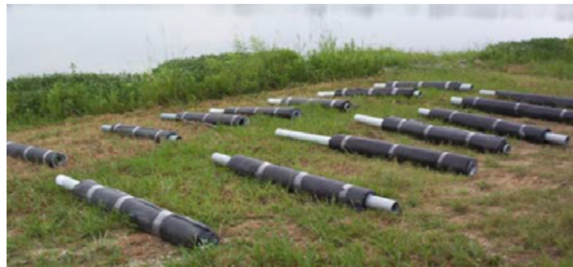
Figure 10. Reactive Mat Material Prior to Deployment at Cottonwood Bay Study Site (Courtesy of SERDP)
