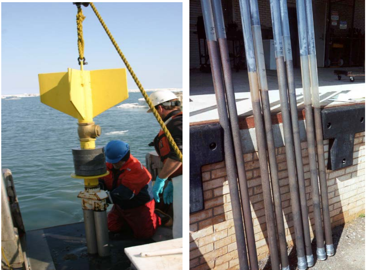
Figure 2-7. Sediment Corer and Collected Sediment Cores in Core Liners
