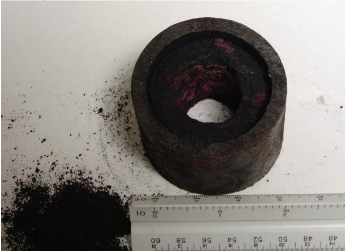
Figure 2. Manganese and related mineral deposition in a groundwater extraction system at Sierra Army Depot.
