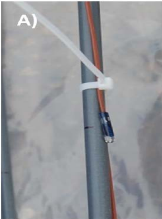
Thermocouple on temperature monitoring "stick"
