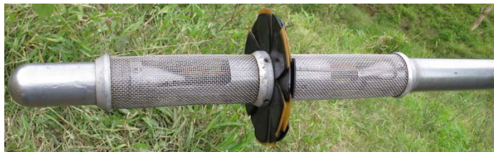
Heat pulse flowmeter – flexible baffle and flow measurement (screen) interval
