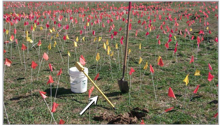
Figure 1. Example of the magnitude of the cleanup when all metal objects in the subsurface require removal by digging. Sensor shown is a non-AGC metal detector (Courtesy of Defense Science Board, 2003).
