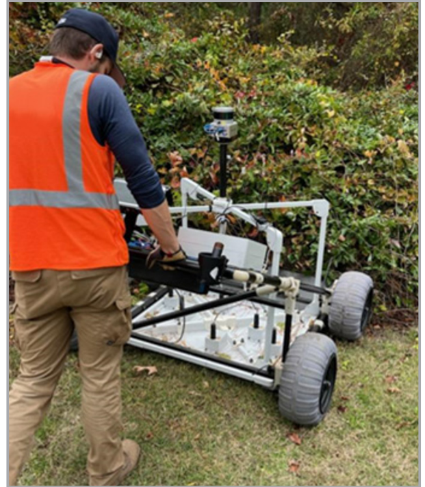
Figure 3. Operation of a one-pass AGC sensor at a DoD facility (Courtesy of Jacobs).
