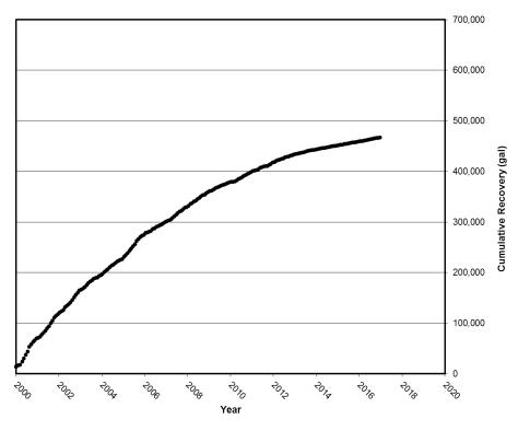
Figure 3-2. Cumulative LNAPL Recovery (Courtesy of NAVFAC)
