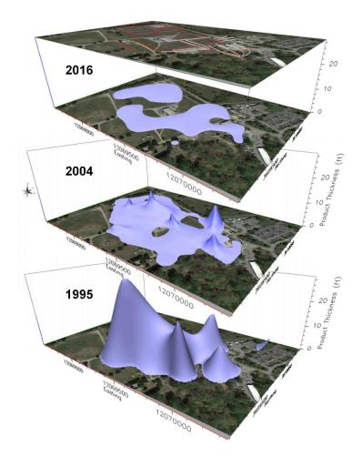
Figure 3-4. Reduction of LNAPL in Monitoring Wells (Courtesy of NAVFAC)
