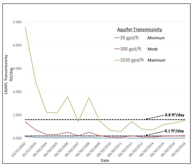
Figure 3-3. LNAPL Transmissivity as a Function of Time (Courtesy of NAVFAC)
