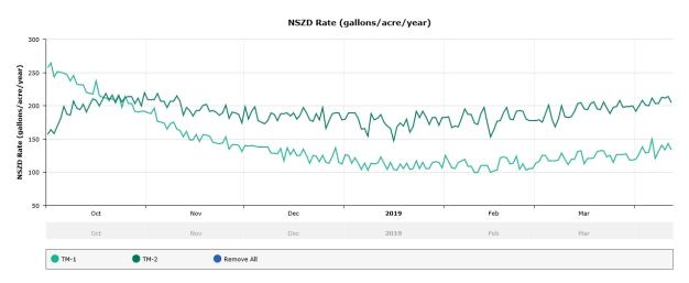
Figure 3-10. Measured Daily NSZD Rates (Courtesy of NAVFAC)
