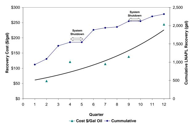
Figure 2-3. Normalized Cost of a Multiphase Extraction System at Site 6, Naval Construction Battalion Center Gulfport (Courtesy of NAVFAC)
