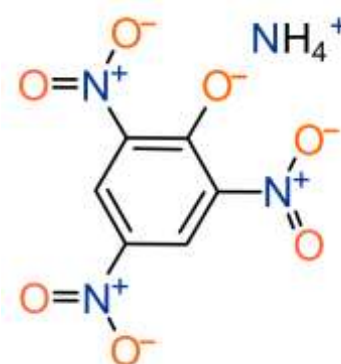
Figure 18-1. Chemical Structure of Ammonium Picrate
