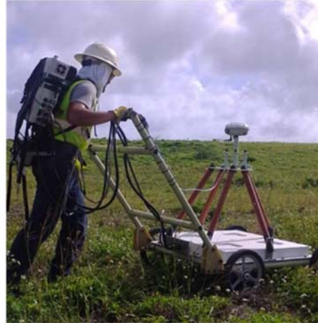
Figure 4-13. Smaller, more portable versions of AGC sensors: MPV (left) and MetalMapper2X2 (right)
