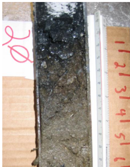
Figure 2-3 Split Soil Core Shows Minimal Natural Mixing of AC into BAZ has Occurred at Time 0
