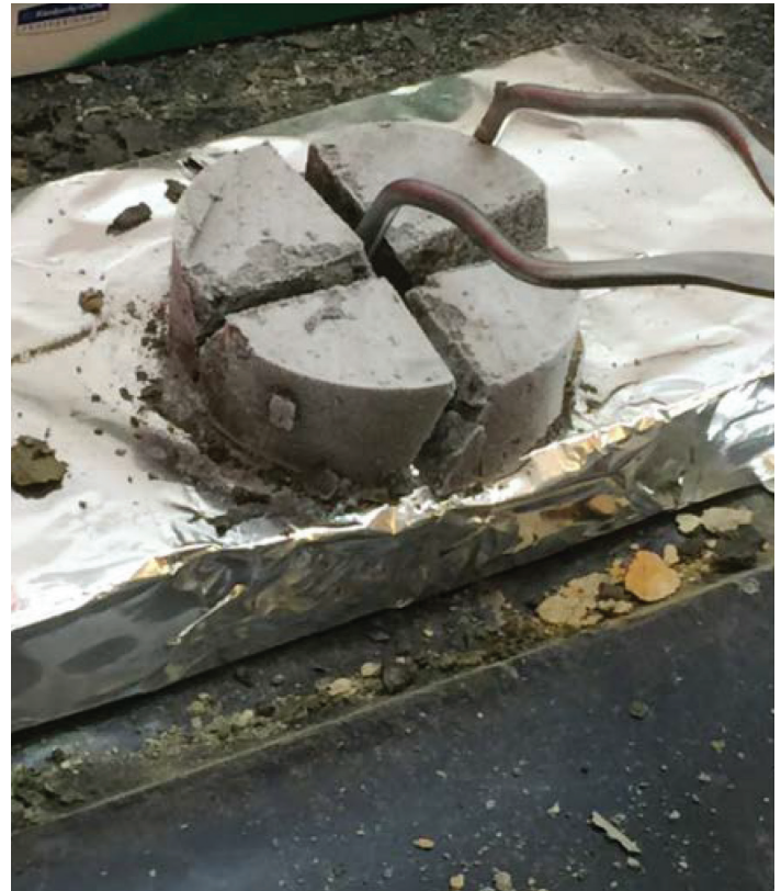
Figure 6. Processing Soil Cores Collected by Cryogenic Coring (Courtesy of ESTCP)
