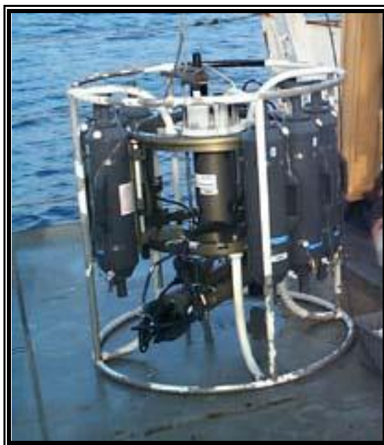
Figure 8-2. Hydrocast Surface Water Sampling Device.
