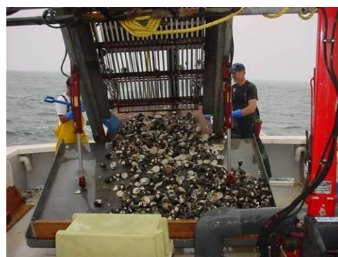
Figure 10-4. Shellfish Sampling Using Commercial Hydraulic Dredge (Photo Courtesy of Battelle Ocean Sciences Laboratory)
