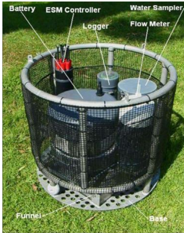
Figure 8-4. UltraSeep® Surface Water Sampling Device (Source: RITS on Coastal Contamination Migration Monitoring, NAVFAC ESC, 2003)
