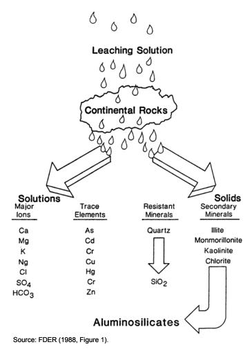
FIGURE 2-4. Conceptual model of the chemical weathering process
