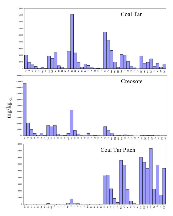
**Figure A-4. Histograms of selected pyrogenic sources.** For PAH compound abbreviations, see Table A-2.
