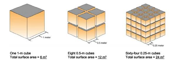
As a cube is divided into smaller units, the volume remains unchanged, but the overall surface area increases.
