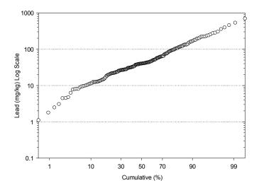
FIGURE 2-19. Log-scale probability plot of lead concentrations (background)
