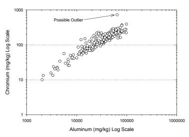
FIGURE 3-3. Scatter plot of chromium vs. aluminum concentrations (log scale) showing strong association
