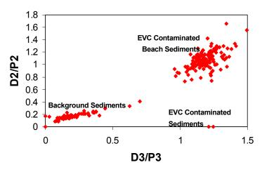
FIGURE A-12. Cross-plot of dibenzothiophenes and phenanthrene concentrations in Prince William Sound sediments. EVC – ExxonValdez cargo. (Source: Page et al., 1996.)
