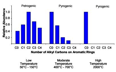
FIGURE A-2. Representative distribution of alkylated PAHs formed at different temperatures (after Blumer, 1976)
