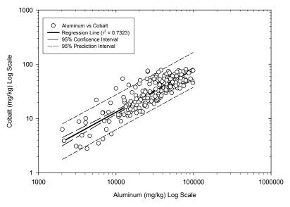
FIGURE 5-7. Geochemical regression: cobalt vs. aluminum
