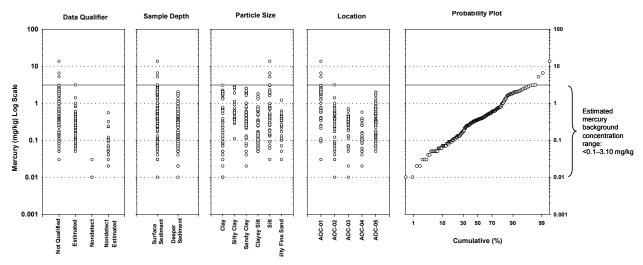
FIGURE 2-21. Combined mercury plots (univariate and cumulative probability)
