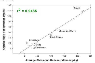
FIGURE 2-6. Correlation plot of nickel vs. chromium concentrations
