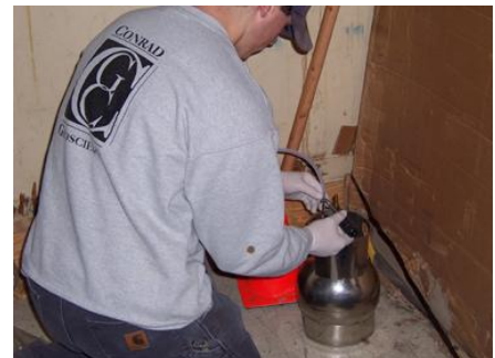
Indoor air sampling was conducted in January 2009 in homes along 11 th Street. Results indicate elevated levels of TCE in the indoor basement air of several of the homes sampled.
