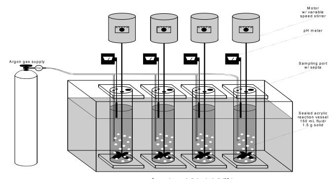
Temperature-controlled water bath (373C)
