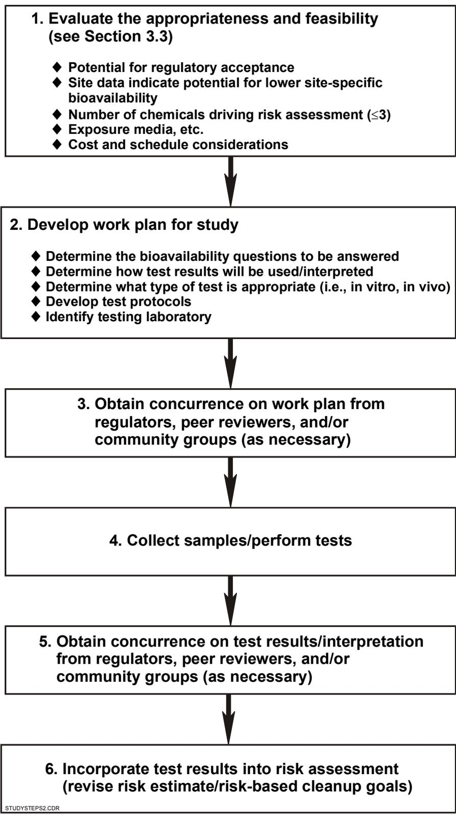
**Figure 4-4. Steps in Conducting a Bioavailability Study**
