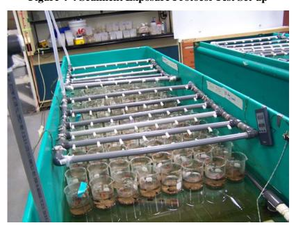
Figure 4-4 Sediment Exposure Protocol Test Set-up
