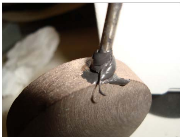
Figure 1 – Photograph of the temperature monitoring disc for red mudstone with a thermocouple placed inside the drilled hole to monitor the temperature profile in the disc during the heating tests.
