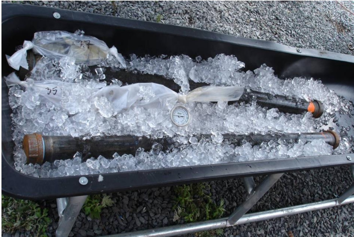
Figure 5.27. Core Barrels Containing Hot Bedrock Being Cooled Before Rock Sampling
