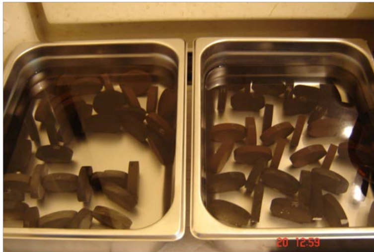
Figure 2 – Photograph of the red mudstone, gray mudstone and black mudstone disc samples under TCE saturation at the left, and PCE saturation at the right.
