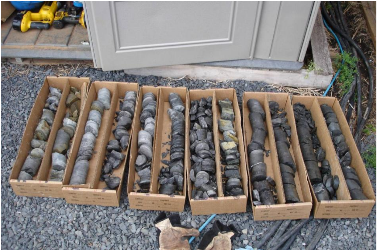
Figure 5.29. Pre-Treatment Rock Cores
