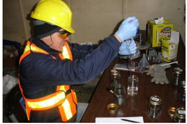
Figure 5.28. Cutting and Methanol Preservation of the Cores
