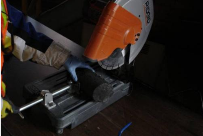
Figure 5.28. Cutting and Methanol Preservation of the Cores
