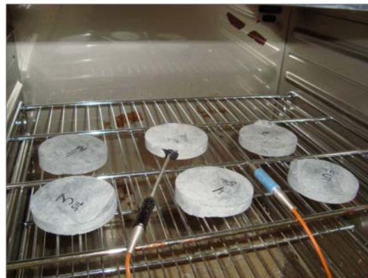
Figure 3 – The distribution of the set of TCE saturated siltstone discs, the temperature monitoring disc and the extra thermocouple inside the convection oven.
