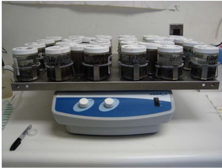
Figure 6 – Photograph of the orbital shaker where the TCE and PCE extracts remained for 24 hours to attain complete extraction of VOCs.
