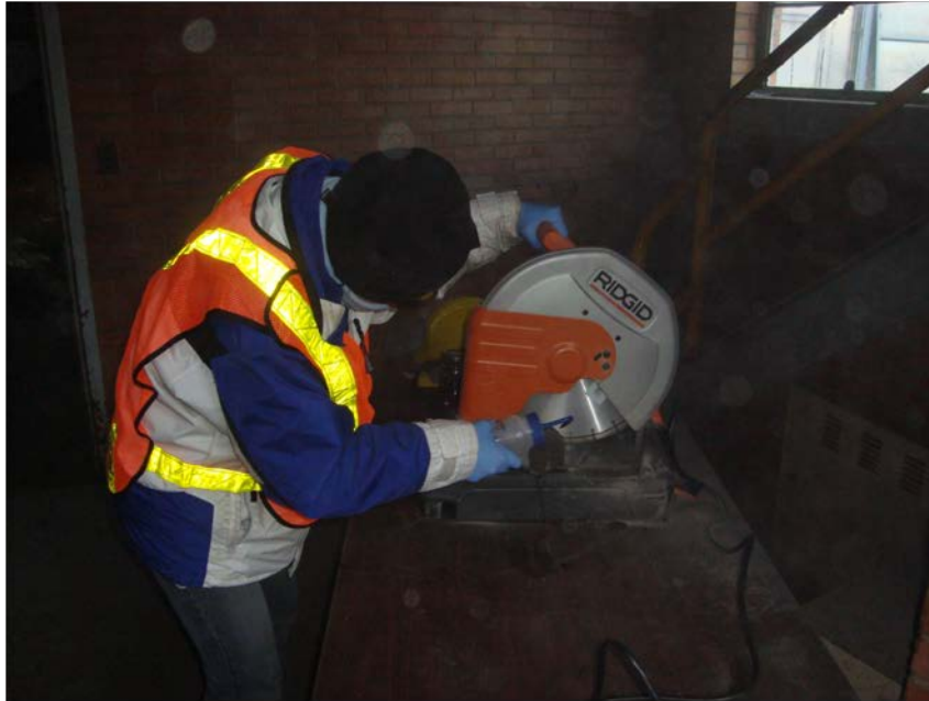
Figure 2 – Photograph of the cutting of the 1 cm thick discs from the recollected rock core at the NAWC site.
