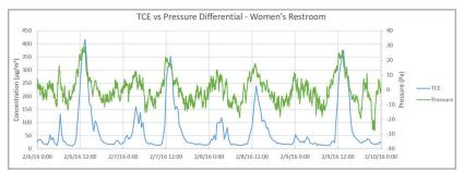
Figure 3. TCE Monitoring Results by ECD and Pressure Differential (Courtesy of Battelle)
