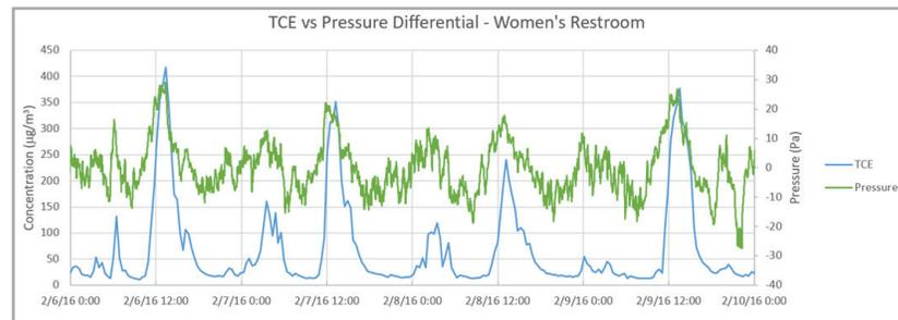
Figure 3. TCE Monitoring Results by ECD and Pressure Differential (Courtesy of Battelle)
