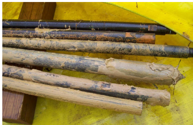
Figure 4-3. Clogged Injection Tooling
