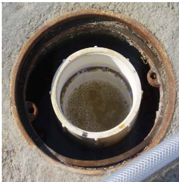
Figure 3-3. Gas Generation during Application of Iron-Activated Hydrogen Peroxide
