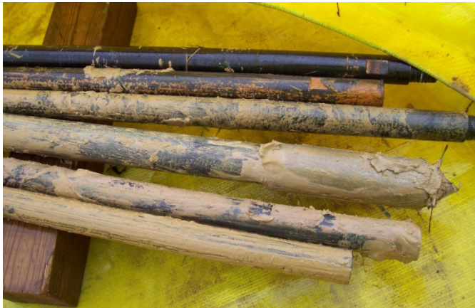
Figure 4-5. Clogged Injection Tooling
