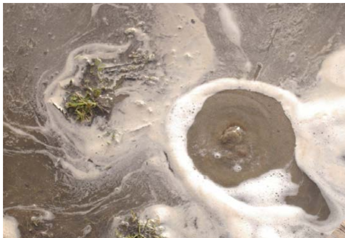
Figure 4-8. Surfacing of Groundwater during Application of ISCO Using Iron-Activated Sodium Persulfate
