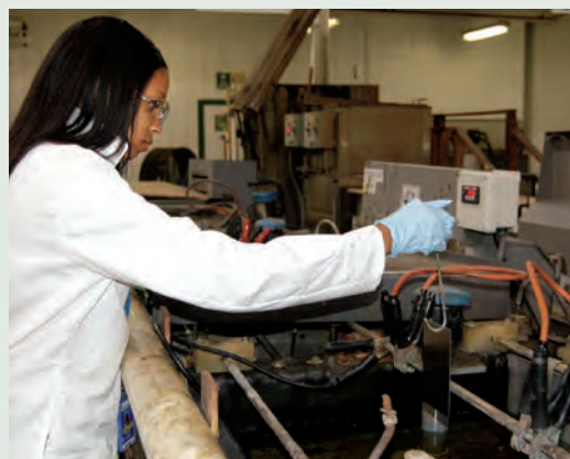
Under this NESDI project, Kami Downey (shown here) devised a silver electroplating and strip process that removed cyanide from the waste stream. (Photo Credit: Victor Pitts)
