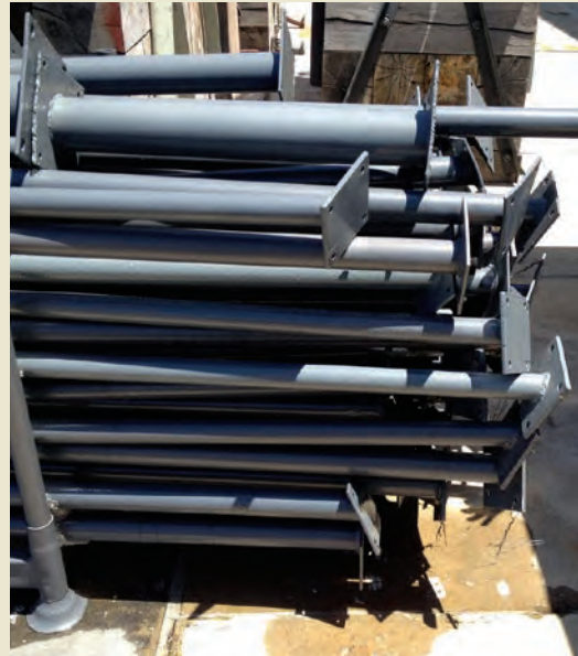
Galvanized metal is one of the major sources for zinc runoff in stormwater. (Photo Credit: Chuck Katz)
