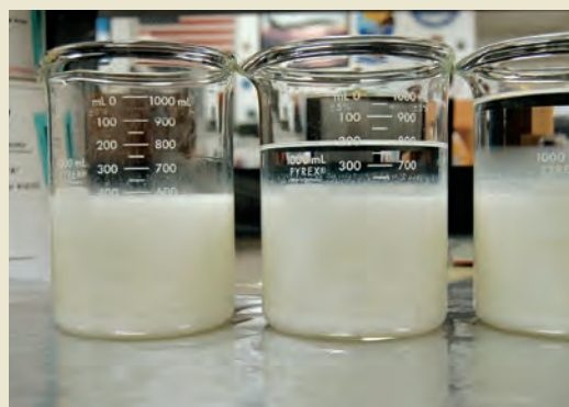
The D-Zolve product without an oil seal, with a 200 milliliter (mL) oil seal, and with a 400 mL oil seal.
