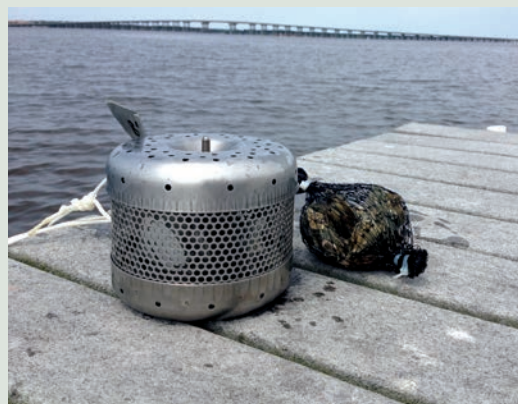
The POCIS encased in its canister.
