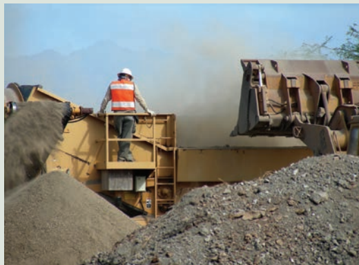
Dewatered excavated dredged material being screened for MEC. Photo by Fred Goetz
