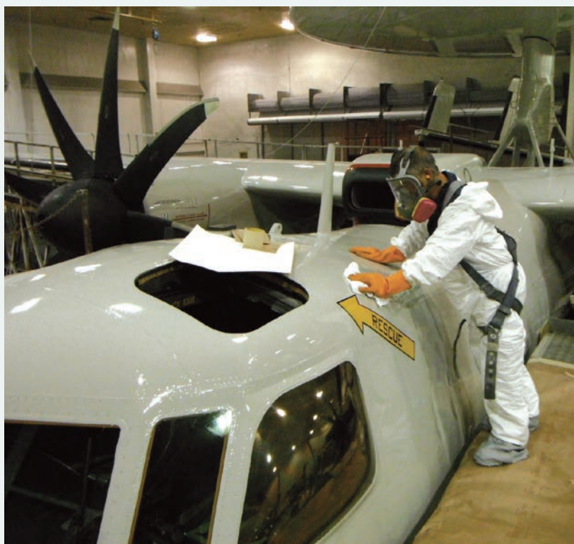
Worker applies new low-VOC solution. Photo by Luc Doan
