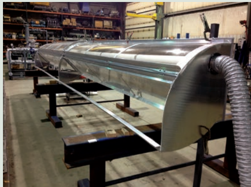
The prototype capture system. Photo by Jim Howell
