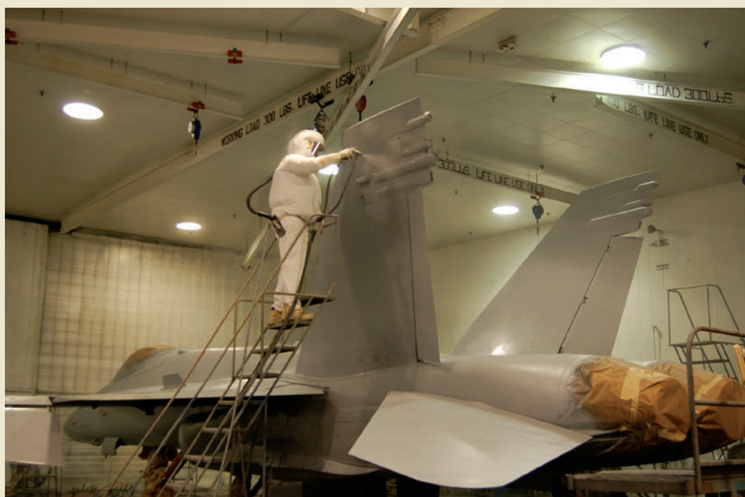
Worker applying polyurethane coating to an F/A-18 aircraft. Photo by Jennifer Nunez
