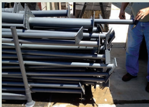
Galvanized metal contributes to metals loading in stormwater runoff. Photo by Chuck Katz
