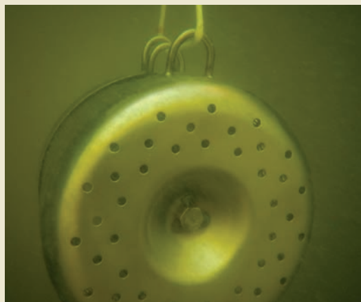
A Polar Organic Chemical Integrative Sampler (POCIS). Photo by Gunther Rosen
