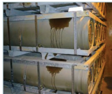
Epi-Seal leakage on stored bombs.
