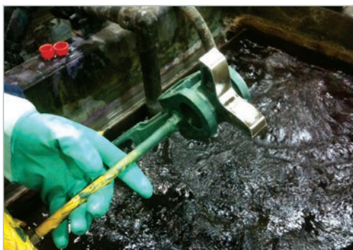
nCoP-treated T-45 part (project 348).
