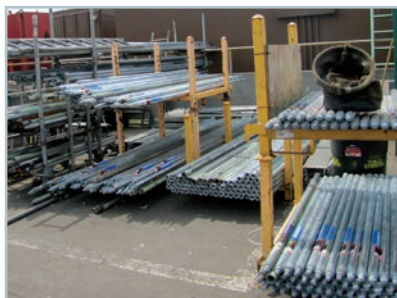
Galvanized metal pipes contribute to metals loading in stormwater runoff.
