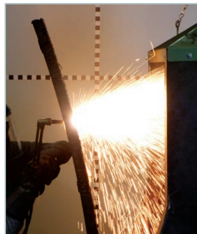
The hot cutting process on a submarine hull sample. Jim Howell
