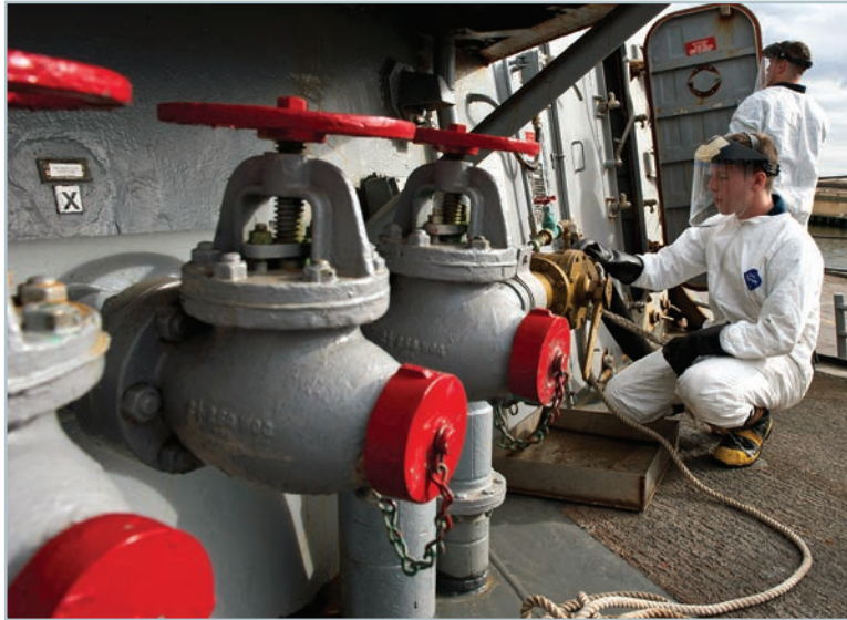
Sailors aboard the Arleigh Burke-class guided-missile destroyer USS Porter (DDG 78) disconnect the CHT system from shore drainage while preparing to get underway. MC Specialist 3rd Class Scott Pittman
