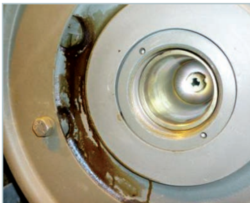
Leaked Epi-Seal material on the aft surface of a 2,000-pound general purpose bomb. U.S. Air Force
