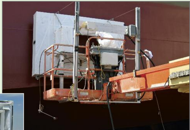
The MAEE can be assembled on a conventional boom lift in approximately one hour.
