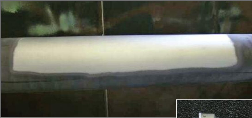
Composite antenna mast from Pearl Harbor Naval Shipyard after CHP stripping.
