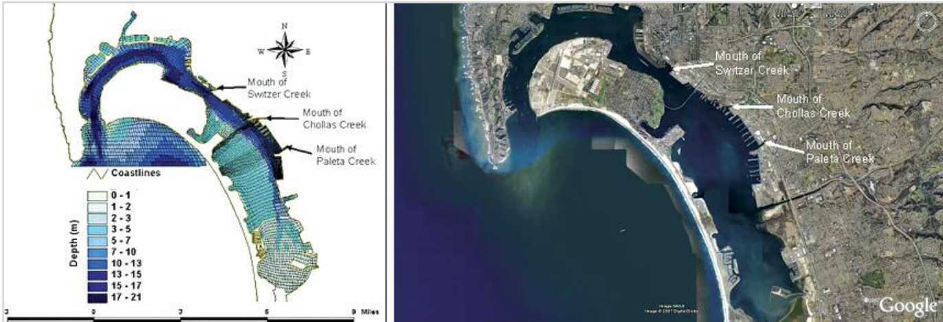
Model grid for the linked CH3D+GNOME model for San Diego Bay with variable grid sizes.
