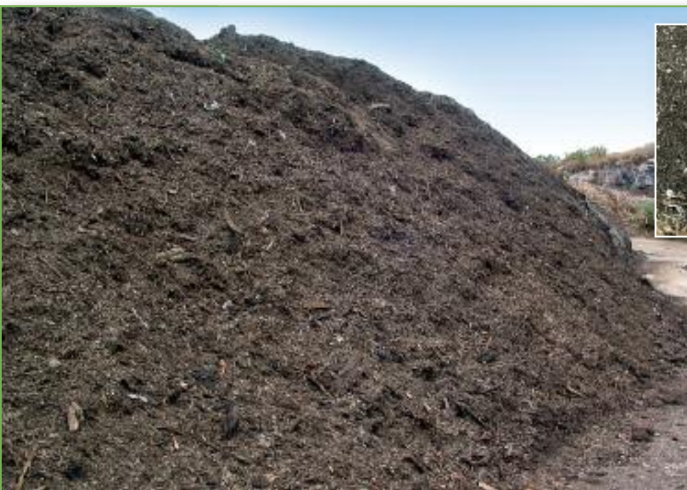
Compost amendment added to raw dredge material.
