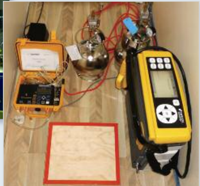
A traditional method of sampling sub-slab air includes the Inficon Hapsite® system used with conventional Summa canisters and verification of air pressure difference between in-floor and sub-slab.
