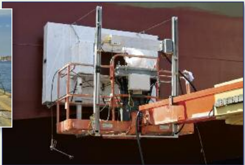
The MAEE can be assembled on a conventional boom lift in approximately one hour.
