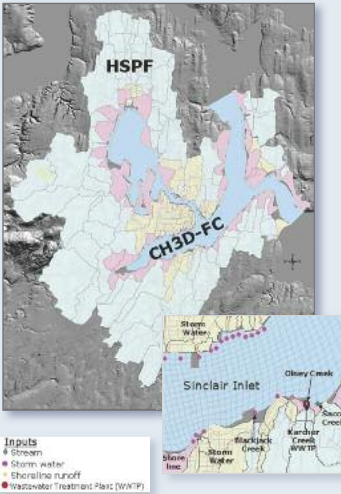
Map of the Sinclair and Dyes Inlets showing streams (green watersheds), shorelines (pink watersheds), and stormwater outfalls (yellow watersheds) modeled by HSPF; the numerical grid of the receiving waters modeled by CH3D-FC, and detail of model inputs (inset).
