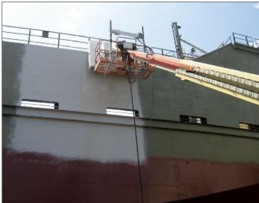
The MAEE control system's micro-computer converts the operator's instructions into precise commands that follow along the ship's hull.
