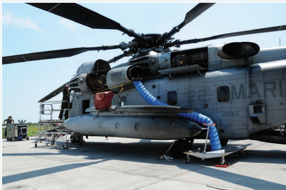
This NESDI project is demonstrating a new engine washing procedure for use across NAVAIR. Shown here is an H-53 helicopter engine wash demonstration with the EcoPower small wash unit and effluent collecting kit in place.
