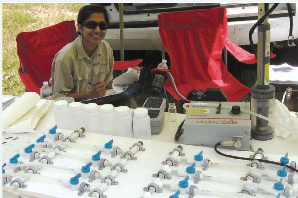
Real-time multi-level monitoring of remedial amendment injection.
