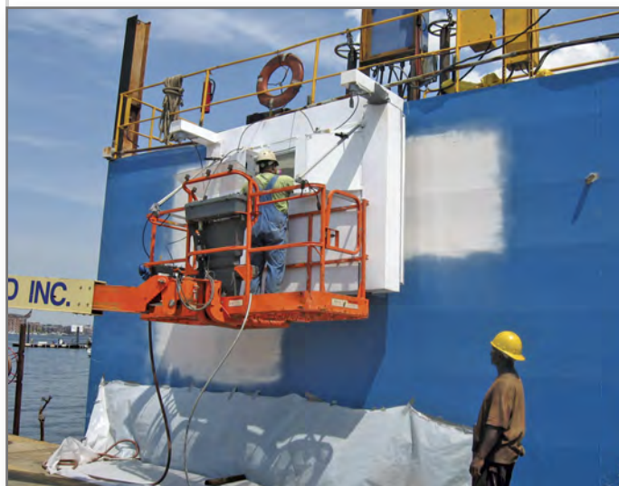
The control system's micro-computer converts the operator's instructions into precise commands that follow along the ship's hull.
