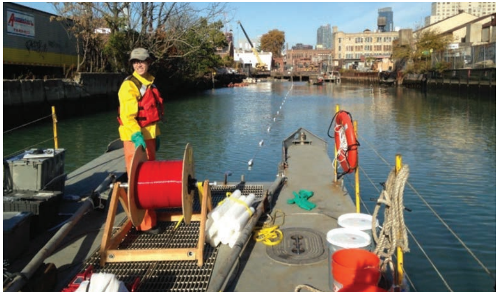
Deployment of the distributed temperature sensing system. (Photo Credit: Joey Trotsky)
