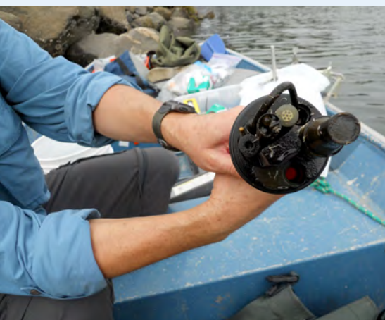
Close up of a dissolved oxygen sensor covered by algae.
