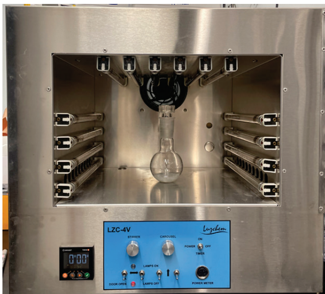
Flow reactor that will be used in the demonstration of photocatalytic degradation of PFAS. (Photo credit: Patrick Fedick, PhD)
