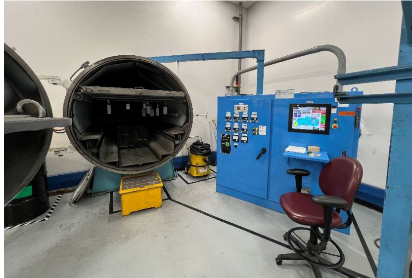
Ion Vapor Deposition (IVD) vacuum chamber is used for the application of aluminum coatings onto substrates which result in higher temperature resistance and a safer alternative to hexavalent chromium coatings. (Image Credit: Kaitlyn Elkins)
