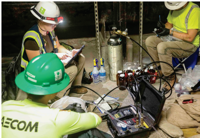
Contractors performing groundwater sampling at a remediation site. Highly specialized training and equipment is used to collect ground water samples. (Image Credit: U.S. Navy photo by Mass Communication Specialist 1st Class Glenn Slaughter).
