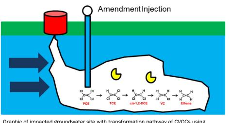
Graphic of impacted groundwater site with transformation pathway of CVOCs using bioaugmentation (amendment injection of dechlorinating bacteria). (Image credit: Tony Danko)
