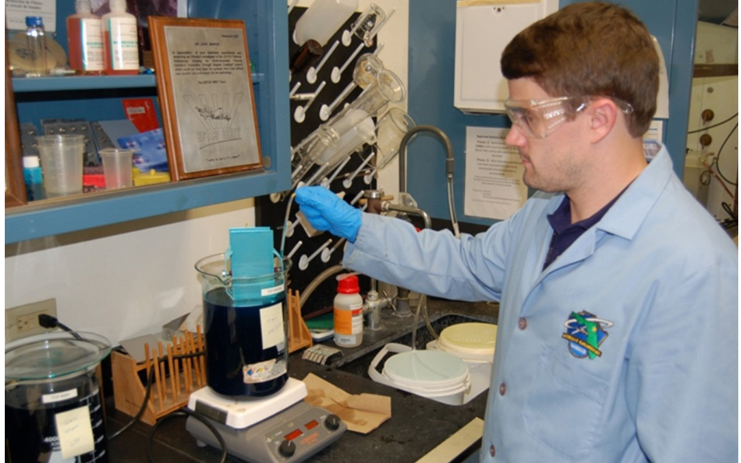
Principal Investigator Sheridan from NESDI project 514 conducts an initial trivalent chromium pretreatment. This project will test the product developed under this project along with others.
