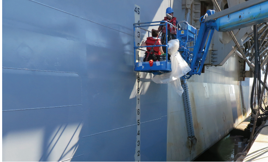
Sailors painting the freeboard of the USS Essex (LHD-2) with single-component polysiloxane topcoat. (Photo Credit: Erick Iezzi)
