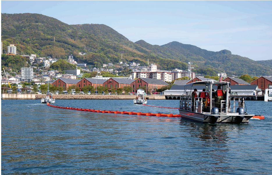
Sailors conduct facility response training which includes a simulated oil spill and oil spill recovery using two utility boats, a dedicated skimmer boat and oil booms to contain the spill. Alternative skimming technologies would greatly reduce the number of manhours required for spill cleanup. (Photo Credit: Seaman Jasmine Ikuseibiala)
