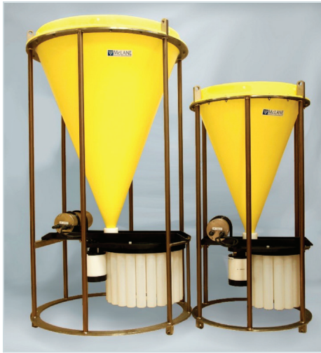
Two different sizes of a time-series sediment trap. (Photo Credit: Courtesy of McLane Research Laboratories.)
