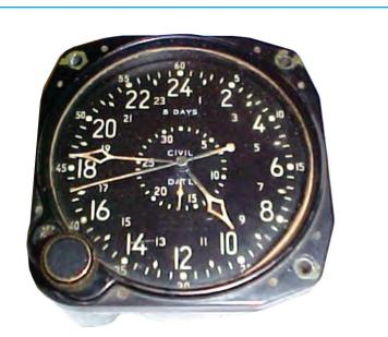
Radium painted dials like the one on this ship's clock can contain small, usually microscopic, radioactive particles and are sometimes found in the marine environment at Department of Navy locations. (Photo Credit: Jovan Popovic)
