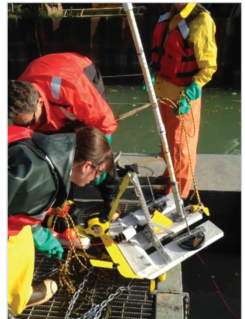
Submersible plow used to bury DTS cable below sediment surface. (Photo Credit: SelkerMetrics)
