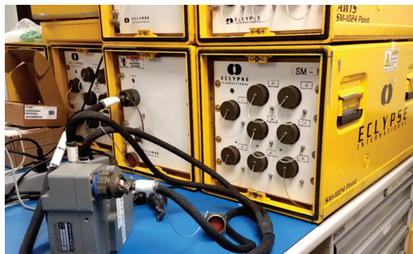
The V-22 Osprey Automated Wiring Test Set (AWTS) will act as the test bed for this NESDI project.
