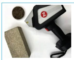
The LIBS analyzer will be used to measure contaminants on urban/industrial surfaces and within soils. (Photo Credit: Patrick Sims)
