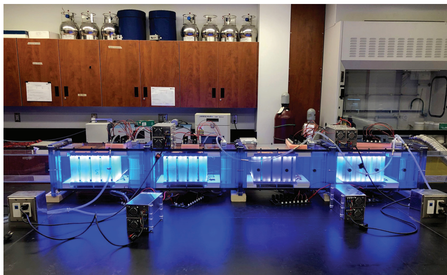
SmogStop prototype photocatalytic oxidation filter testing in the laboratory.
